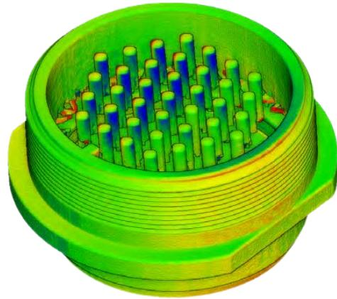
*This printed electrical connector is accurate to the original CAD design, with a 4 sigma tolerance value of +167/-123 microns*
